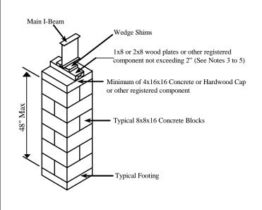
Pier B: Interlocked double stack of solid or open cell 8x8x16 concrete blocks. The maximum height is 48 inches as measured from the top of the footer to the top of the last concrete block. Piers of greater heights are allowed if they are within limits established in adopted federal standards. The pier is capped with a minimum 16x16x4 concrete cap. Open cells must be vertical and in alignment. Each course of open cell blocks must be perpendicular to the previous course.
