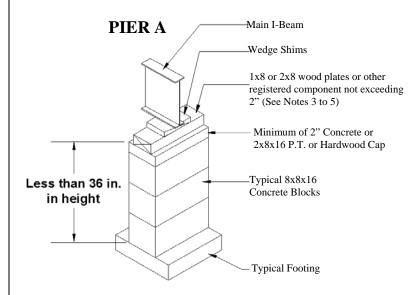
Pier A: Single stack of solid or open cell, 8x8x16 concrete blocks. Maximum height is 36 inches as measured from the top of the footer to the top of the last concrete block. Concrete blocks are installed with their lengths perpendicular to the main I-Beam. Open cells must be vertical and in alignment.
